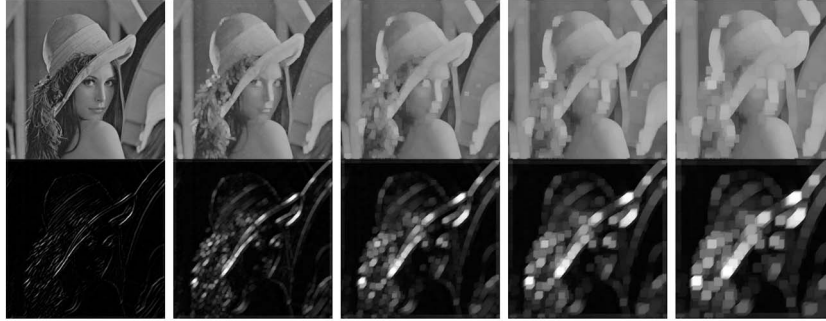
Fig. 11. Max scale space images of Lena (top row) and of the Gabor filtered version of Lena (bottom row). While the gray-value image gets distorted, the information in the sparse edge image is enhanced.
